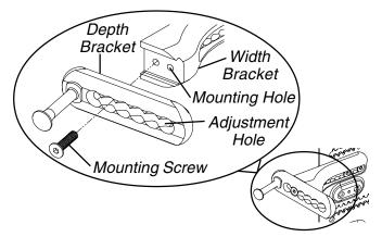
FIGURE 4 - ADJUSTING THE DEPTH HARDWARE
